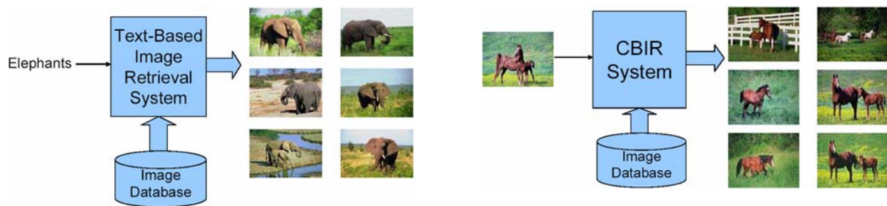
Figure 1: Scheme diagrams of a text-based image retrieval system (left) and a content-based image retrieval system (right).
